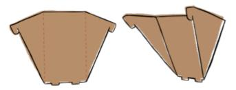
3 Align the slots at the base of the support piece with the slots at the base of the legs [1][2] (furthest from the table top [3]). Simultaneously align the tabs at the top of the support piece with the slots at the top of the legs (closest to the table top)
