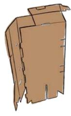
③ Slot the tabs shown below into their corresponding cutouts. All tabs should stick through and be visible on the other side
