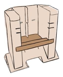
© Repeat steps 1–5 for the second shelf, using the remaining slots closer to the feet of the legs
