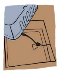
Seat the ChompSaw into the insert[6] - it should fit just right
