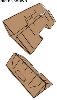
⑤ Grab the assembled left leg [1] and slot it into the table top as shown
