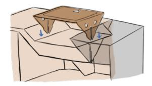
When the insert is almost fully inserted, guide the tabs on the insert into the slots on the underside of the table top
