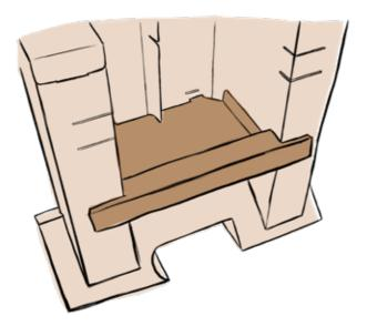
When the shelf is almost fully inserted, take care to guide the shelf tabs into the slots at the back of the legs
