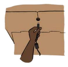
③ Plug the power supply's barrel jack plug into the ChompSaw's barrel jack recepticle
