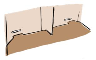
Fold up the shelf lip, slotting the tabs on the folded lip into the corresponding cutouts on the legs
