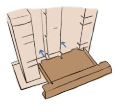
The shelf slot should also line up with the leg slot shown in the center below
